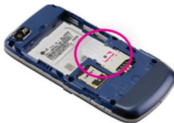
4. Align the gold contacts on the battery with the contacts in the battery compartment. Push the battery into place and replace the battery cover.
